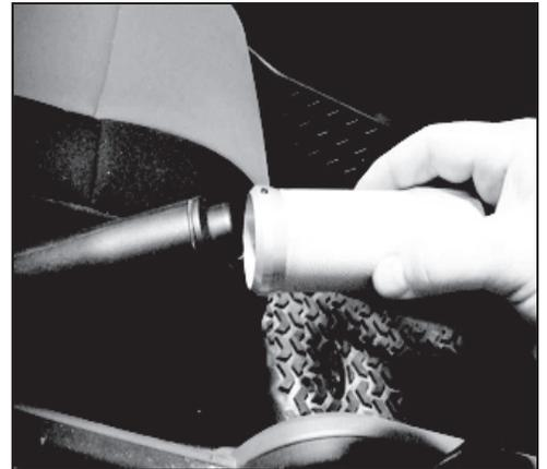
Step 2. Tighten both Allen head set screws. Do not overtighten. Test emergency brake handle to ensure proper function before operating vehicle.
