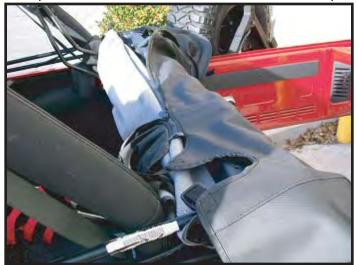
2. Pull the sides of the boot tight and insert the lip into side retainers on both sides of the jeep.
