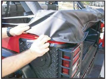
3. Fasten the straps around the roll bar and tighten.
