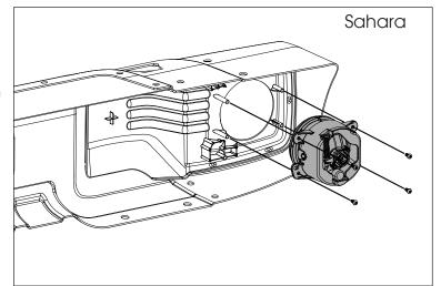
Rubicon Models: Cut inner plastic bosses along shown line using dremal or hobby knife. Install fog light housing to bosses in Plastic Cover using supplied Thread Forming Screws. Do not overtighten.
