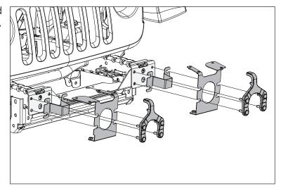
7. Position Bumper Center Section to accept factory Tow Hooks and lower into place on frame rails. Align with holes in Bumper Mount Brackets and loosely attach with M10 Button Head Bolt and Plastic Flat Washers.
