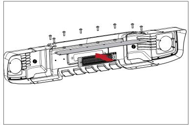
6. Place Stanchion, Bumper Mount Bracket, and factory Tow Hook on frame horns. Using OE Nuts, loosely attach.
