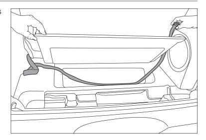
3. Fold back seat down and thread end of seat strap through child seat restraints. Thread strap through buckle and tighten as shown.
