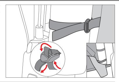
8. Roll plastic strip over edge and into rear groove of body tub. Repeat for opposide side.
