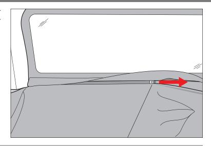
5. Remove tailgate bar from soft top. Insert tailgate bar on tubed strip of tonneau cover and into tailgate mounts on each side of tailgate opening.
