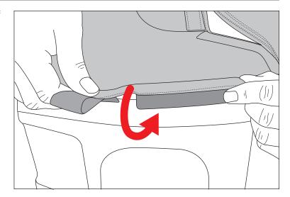
9. Wrap collars around rear sport bar and fasten hook and loop strips together. Repeat for opposite side.
