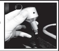
Step 3. Tighten the set screw. Start the vehicle and cycle transfer case into all modes to verify a tight fit. Place transfer case into normal operating position. Test handle to ensure proper function before operating vehicle.
