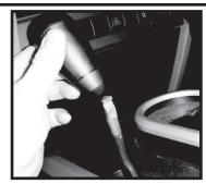
Step 2. Install the new shift knob onto the post. Ensure the shift pattern is orientated correctly.
