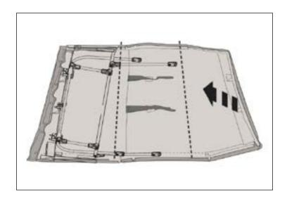
24. **TIP:** It may be helpful to have a second person for this step. Place the top face down and re-fold, beginning with the rear portion.
