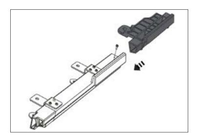
6. Slide Front Rear Bracket onto LH Rear Door Bar as shown below.
