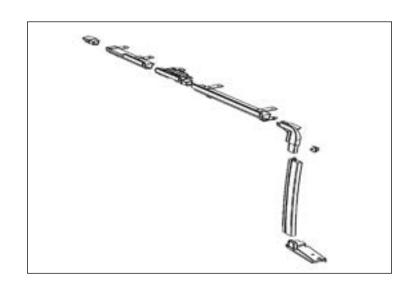
13. Position completed door surround onto the vehicle and fit the bracket over the roll bar.
