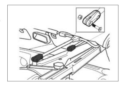
27. Unfold the soft top main deck fabric over the top of the roll cage and in place. Close the top toward the windshield.
