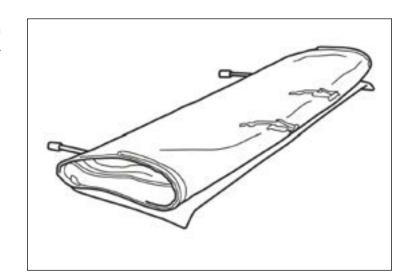
25. Lift the soft top and header channel assembly onto the windshield gasket.
