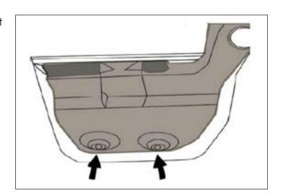
19. Place provided latch as shown and reattach with the screws from the previous step. Do not tighten the screws and adjustment may be needed. Repeat steps 19-20 for the other side.
