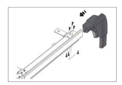
10. Install LH Upright onto LH Upper Corner and secure with Upright Turn Knob.
