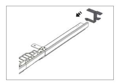
9. Install LH Upper Corner onto LH Rear Door Bar & secure all pieces with 6 self-tap screws.
