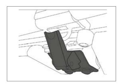
31. Wrap the 2 straps attached to the main section of fabric around the rear-middle of the sound bar. Hook into the holes of overhead brackets. Tighten the strap until snug.
