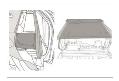
33. Install the hook on rear main straps to the inside of the tub-rail. The hook will slide between the tub-rail and the roll-bar. Now tighten strap.
