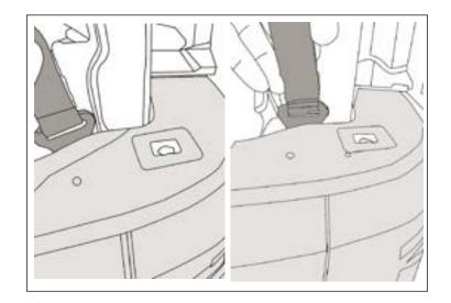
34. Lift up the corners of the top fabric to expose the zippers on the side and rear windows. Secure all windows to the Main Deck by zipping fully into place.
