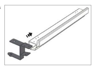
7. Install LH Rear Door Bar onto the adaptor & secure all pieces with 6 self-tap screws.
