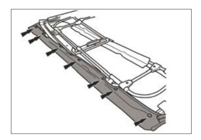
21. Tuck the plastic strip behind latches and along side rails. See photo below for proper fit.
