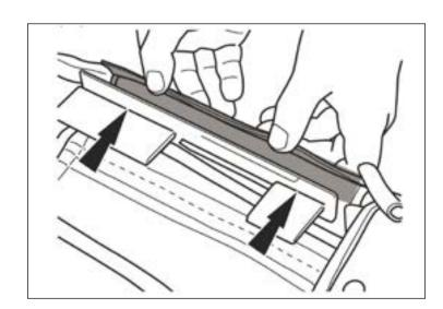
22. Secure the Flip Top Header Assembly to the Soft Top Deck by engaging the Hook and loop flap around the tube.
