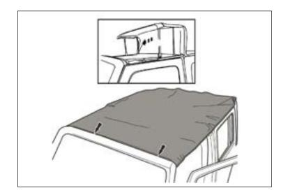
28. Check the front edge to windshield edge lines up to windshield seal.
