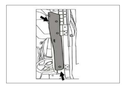
15. Secure the mounting plate to the roll cage using turn-knobs in the holes. Do not fully tighten knob yet.
