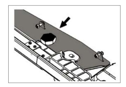
16. Fit top retention strap to driver side - between the hinge plate rear hole and the door surround bracket, and screw down with small knob.
