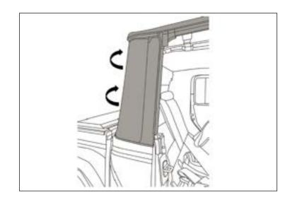
36. Tuck the plastic strip along the bottom edge of the Left Side Window under the Jeep belt rail, by rolling it up underneath the belt rail, beginning at the door, and working your way backward.
