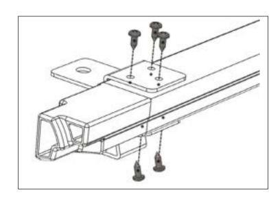
4. Slide Door Surround Front Bracket (Middle) onto LH front door bar and secure with 5 self-tap screws.
