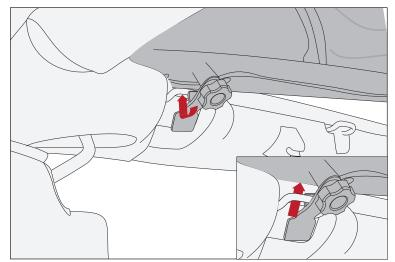
6. Tighten retainer arms by turning threaded lock knobs clockwise. Alternate between the left and right knobs to ensure tight fit.
