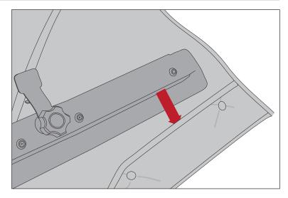
4. Carefully place header and top onto vehicle, ensuring assembly does not scratch or damage windshield. The top and header should rest just behind leading edge of rubber windshield seal.
