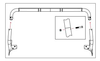
3. Remove the factory LH and RH brackets. Retain factory hardware for later use.
