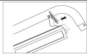
2. Attach LH and RH brackets to crossbar with supplied M8 button head bolt and M8 lock nut. Do not tighten completely to allow for adjustment.
