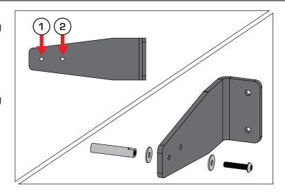
10. Determine correct Striker Plate mounting position. Place Striker Bar in door latch, with mounting flange flush against wall, and fasten to wall using proper fastener for your wall application.
