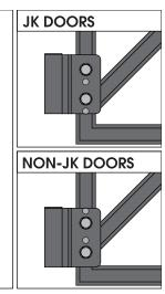
8. Install doors on Wall Mount Door Holder and rest doors against wall.
