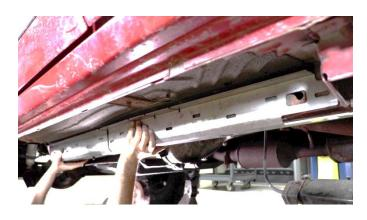
With the help of a friend or a jack, hold the part into place and begin c-clamping it to the rail, away from the bend point.
