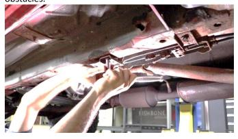
Place a jack or jack stand slightly below the transmission's crossmember, and begin removing the 2 bolts with a 15mm socket. The transmission will fall.
