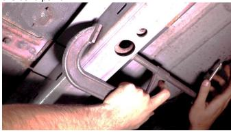
With another jack, press against the part at the bend point, ensuring the steel conforms to the shape of the rail.
