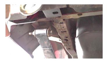
Additionally, if your gas hose cover remains, remove it with a 10mm socket.
