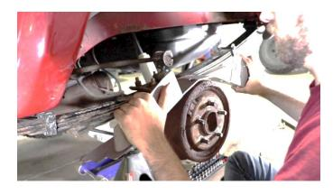
With a jack, push the part up into place, allowing it to bend and conform to the vehicle, while ensuring the holes are aligned. Continue forming the steel along the bend until there are no gaps and clamp it into place. Align the tabs of the bend insert as shown and clamp it into place.
