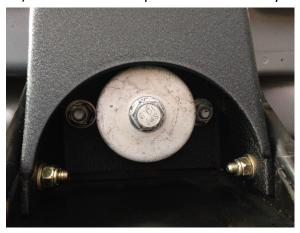
11. The holes now should be drilled 11/32 on each mounting point. Once all mounting points are drilled, debur the drilled holes for a smooth mounting surface.
