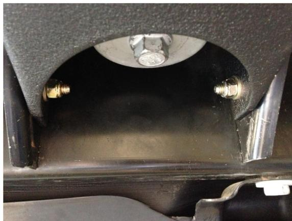
12. Install the 5/16" x 1" bolts, washer & nyloc nuts. Install at the 5 points and torque to 25 ft.-lbs.
