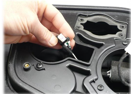
These smaller plugs will stay disconnected and tuck back in their alcoves. You can also tape or tie them so they don't rattle.
