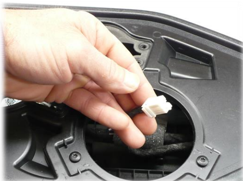
You'll use these larger connectors to mate to the connectors that came with your pods.
