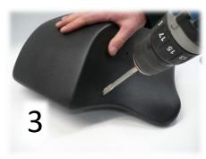
We don't pre-drill wire lead holes so you can put them where you want them. But a good place is the **underside** of each pod (image 2) so there will be no visible wires once installed. With a pod in place, little pieces of tape on the pod and the carpet can act as markers. Remove the pod, then use a 7/16" paddle bit and drill out the hole about an inch in from the edge (image 3). Repeat process in mirror image for other pod. Install the rubber grommets.
