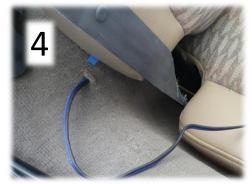
With the tape used as a marker still on the carpet, make a small slit about an inch past the tape so the wire will poke through **under** the pod when it's installed. Run your speaker wire from your radio or amplifier under the carpet and up through slit so about a foot or wire exits. The wire should only be **under** the pod in that tiny area and should be away from the pod after that so you get the best fit. Repeat process for the other pod.
