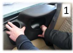
With carpet in it's correct factory position, place a pod on the wheel-well and find the sweet spot by moving it around slightly, but don't screw it in place yet...just get a feel for exactly where it goes.
