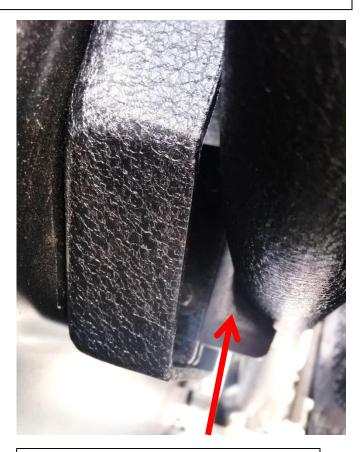
Correct adjustment. No Gap. Tail gate has resistance when closing the last few inches.
