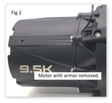
STEP 1: Remove button head bolts, holding down the armor plates on to the motor (Fig. 1), then gently slide the plate to the left to remove it (Fig 2).
