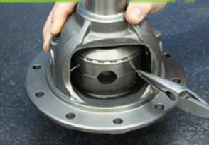
Align the center drivers to correct position & remove retainer wires
