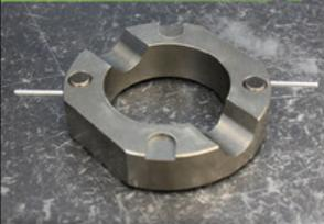
Push alignment pin/spring assembly down & secure with retainer wire
