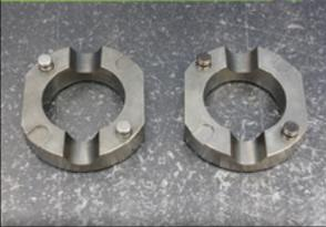
Install alignment pins/springs into driver holes
