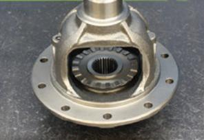
Install side couplers into carrier case
