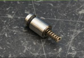
Place springs in hollow end of alignment pins
