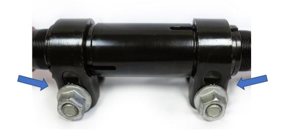
5. THREAD BOTH FORGINGS INTO THE ADJUSTER TUBE. NOTE: WE RECOMMEND USING ANTI-SEIZE ON THE THREADS OF THE FORGING
