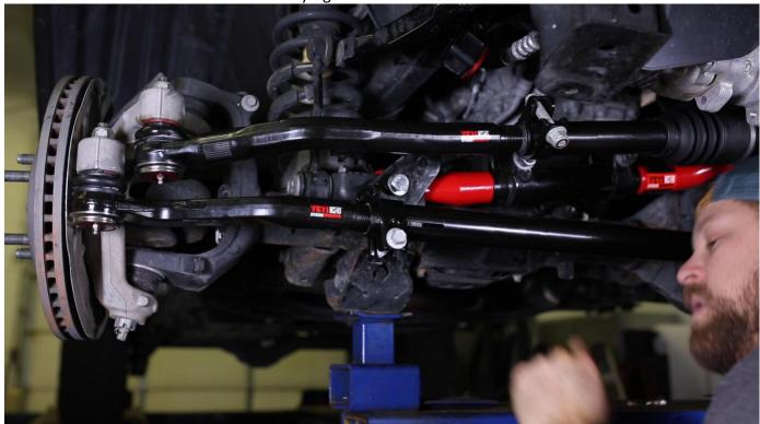
4. Line up/level stabilizer bracket and use center punch to mark center of where you want to start drilling
