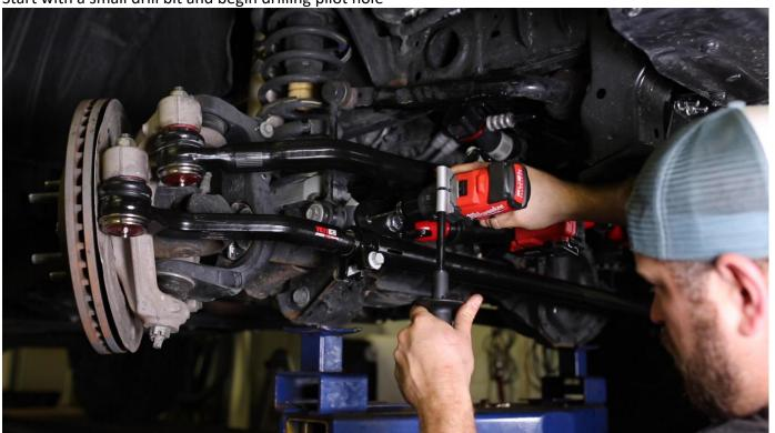
6. Progressively increase the Drill bit size, finishing the hole with a 13/32 (or similar) Drill Bit
