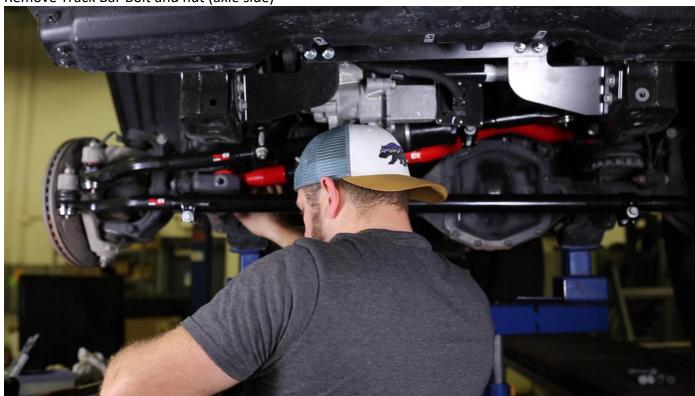
3. Use new M14 fastener and nut and loosely tighten down Stabilizer Relocation Bracket
