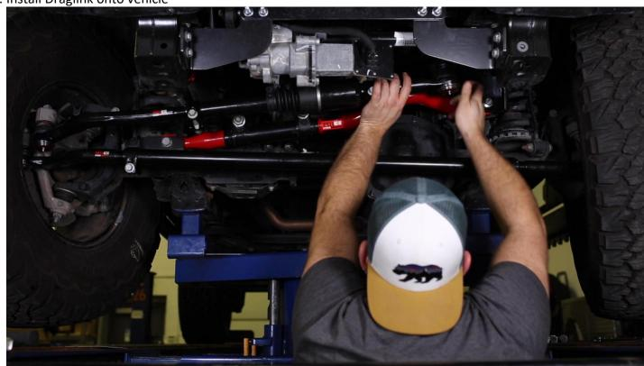
i. Note — clamps still only snugged - you will need to adjust this once everything is back together and the vehicle is on the ground (See Images for correct washer orientation)
