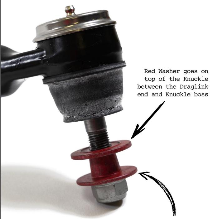
Red Taper Sleeve goes into the bottom side of the passenger steering knuckle
