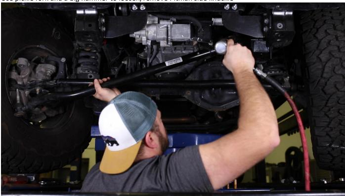
a. We recommended the use of an air hammer with pickle fork attachment for fastest and easiest removal. The joint will be taper locked into the pitman arm and will require a good deal of effort to remove.
