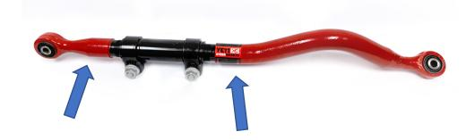
6. MEASURE THE STOCK TRACK BAR FROM THE CENTER OF THE DRIVER BUSHING TO THE CENTER OF THE PASSENGER BUSHING. USE THIS MEASUREMENT TO SET THE LENGTH OF THE NEW YETI XD TRACK BAR. NOTE: TRY TO KEEP EQUAL LENGTHS OF THREAD ON BOTH SIDES OF THE ADJUSTER TUBE.
