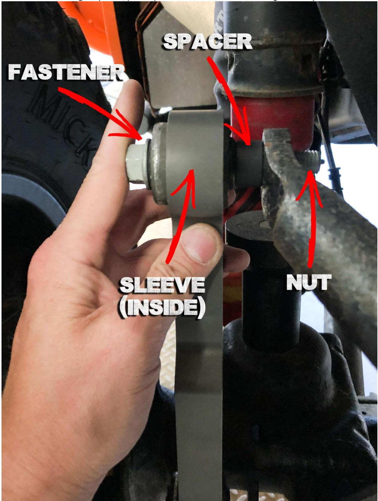
5. Affix M12 nut on the end of M12 fastener and torque to spec.
