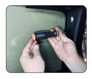
**Step 4**Remove the passenger sun visor by removing the two Torx T20 screws.
