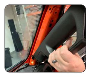
**Step 5**Remove the passenger side sun visor by removing the two Torx T20 screws.
