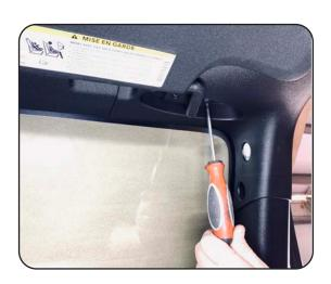
**Step 5**Remove the passenger A pillar trim panel by pulling to release the retaining clips.
