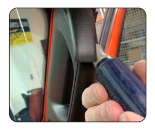
**Step 4**Grasp the handle firmly and pull towards the center of the vehicle to release the retaining clips and remove.
