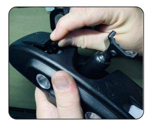
**Step 3**Using a Phillips screwdriver, remove the push rivet from the passenger A pillar.
