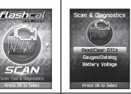
STEP 2 - Select STEP 3 - Select Read/Clear DTCs. Clear DTCs.
