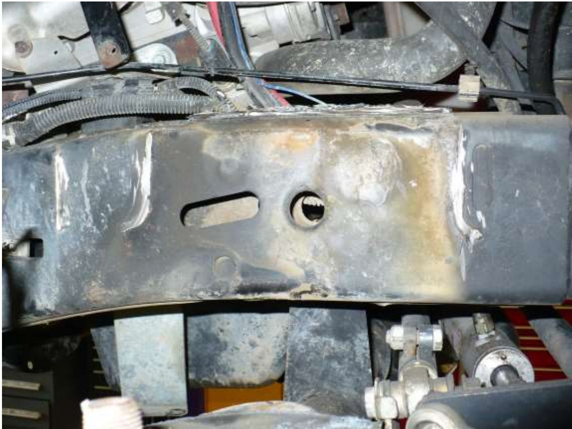
c) Remove the remainder of the coil bracket and grind clean
