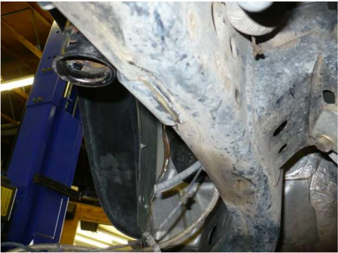
c) Remove the remainder of the coil bracket and grind clean
