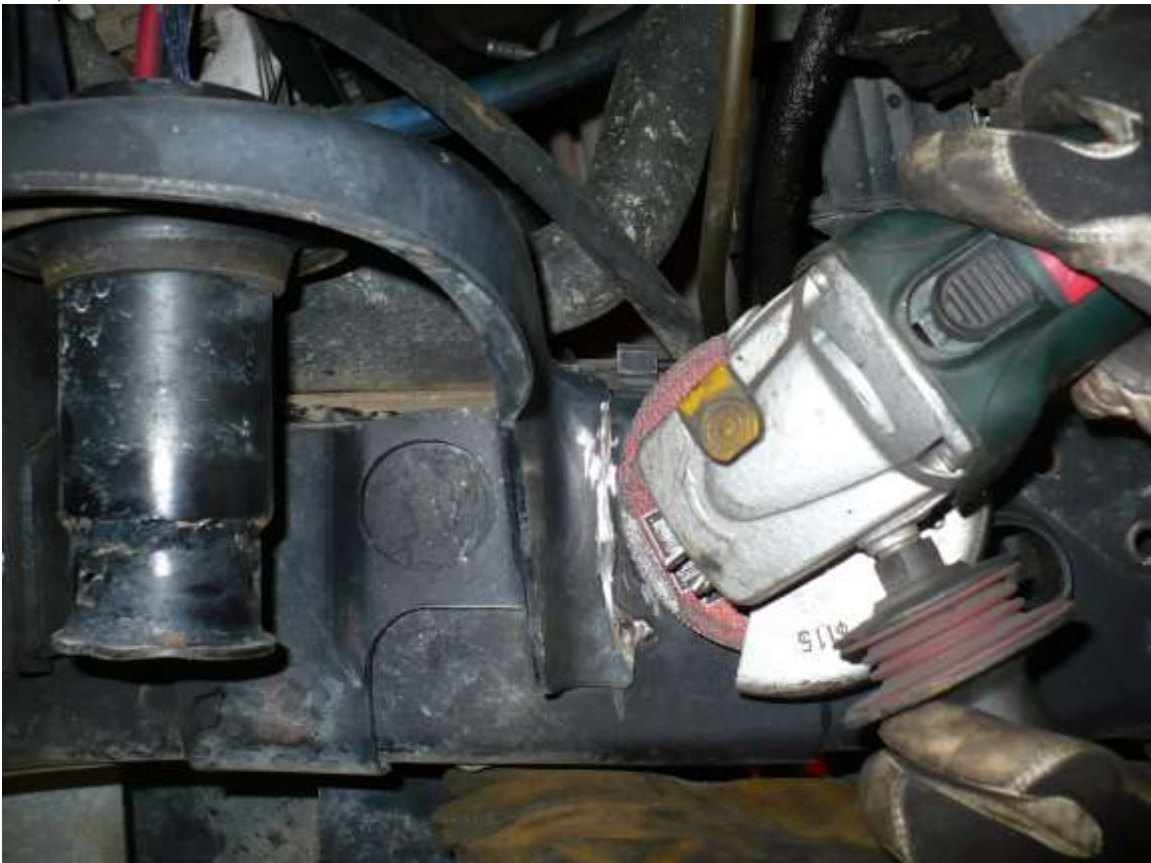
b) Cut the sides and bottom weld that attach the coil mount to the frame
