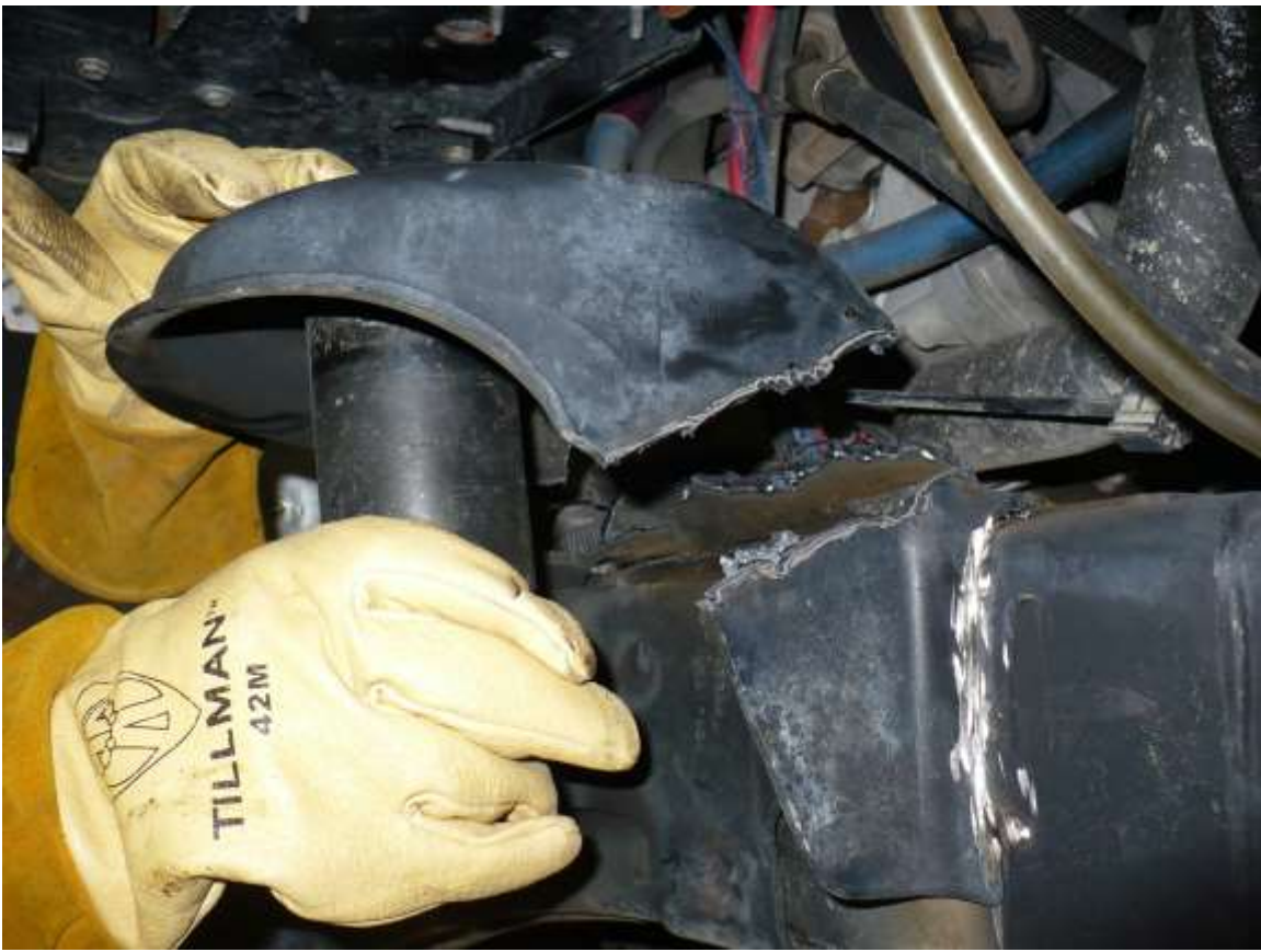
b) Cut the sides and bottom weld that attach the coil mount to the frame
