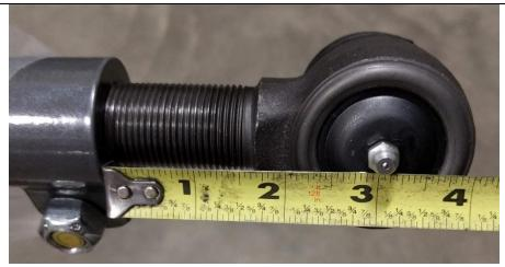
Figure 5. Maximum Length on Non-Double Adjuster (Knuckle) Side
