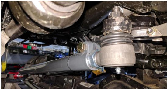
Figure 7. Drag Link Correctly Oriented, Pinch Bolt Up
