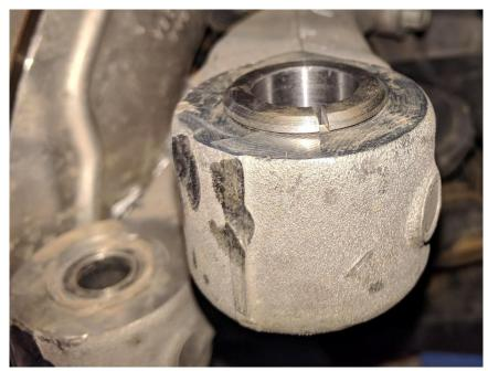
Figure 4. Flip Adapter in Steering Knuckle
