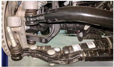
Figure 2. Tie Rod Removed From Knuckle
