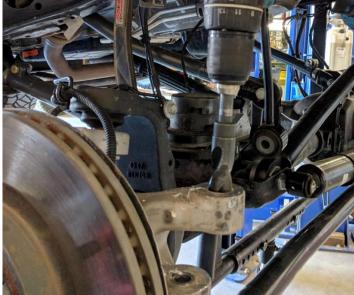
Figure 3. Drilling out Steering Knuckle
