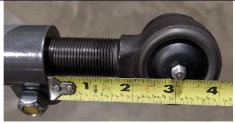
Figure 5. Maximum Length on Non-Double Adjuster (Driver) Side
