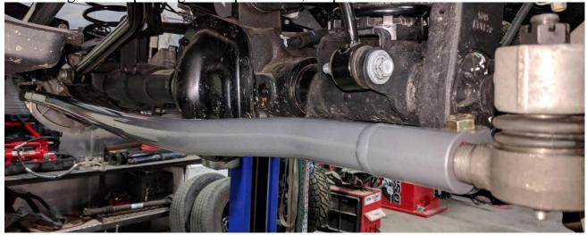
Figure 7. Tie Rod Correctly Oriented, Pinch Bolts Back
