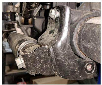
Figure 3. Removing Axle Side Steering Stabilizer Bracket
