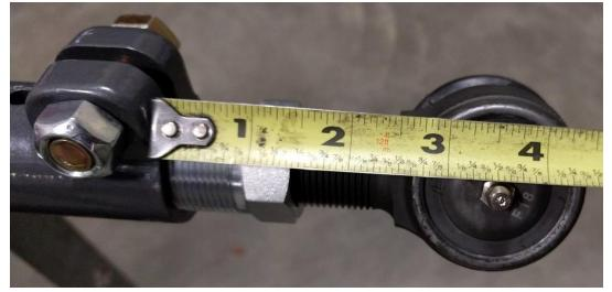
Figure 6. Maximum Length on Double Adjuster (Passenger) Side
