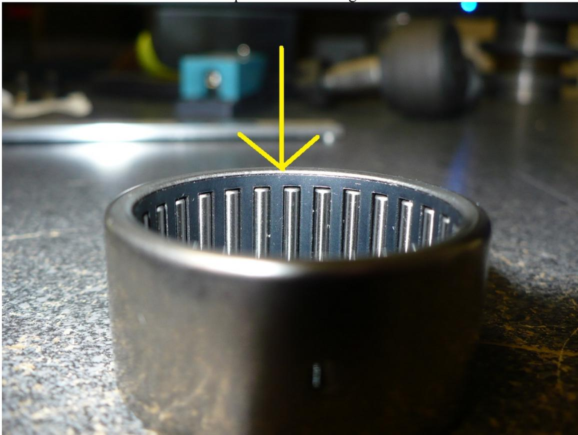
IMG 5.2 – Thinner lip of needle bearing. DO NOT press from this side.
