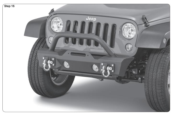
Finally, install D-Rings with provided washers and Isolators. (Step 15)
