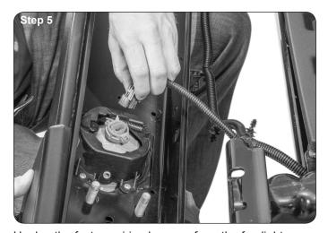
Unplug the factory wiring harness from the fog lights. (Step 5)  $\,$
