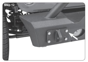
Pass 4 M12 bolts through the D-ring mounting bracket and through the factory frame holes. Repeat on other side. (Step 12)
