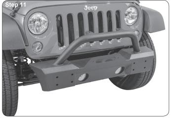
With the help of a friend lift the bumper into place on the frame of the Jeep. (Step 11)
