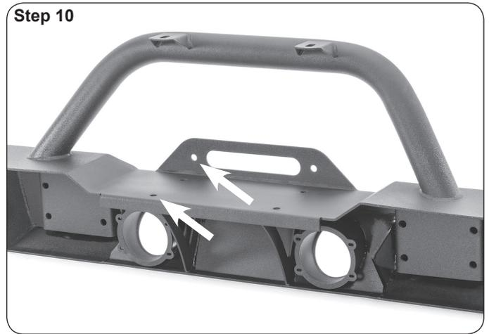
Before installing the bumper you must first install your winch and fairlead on to the bumper according to your winch's installation instructions.
