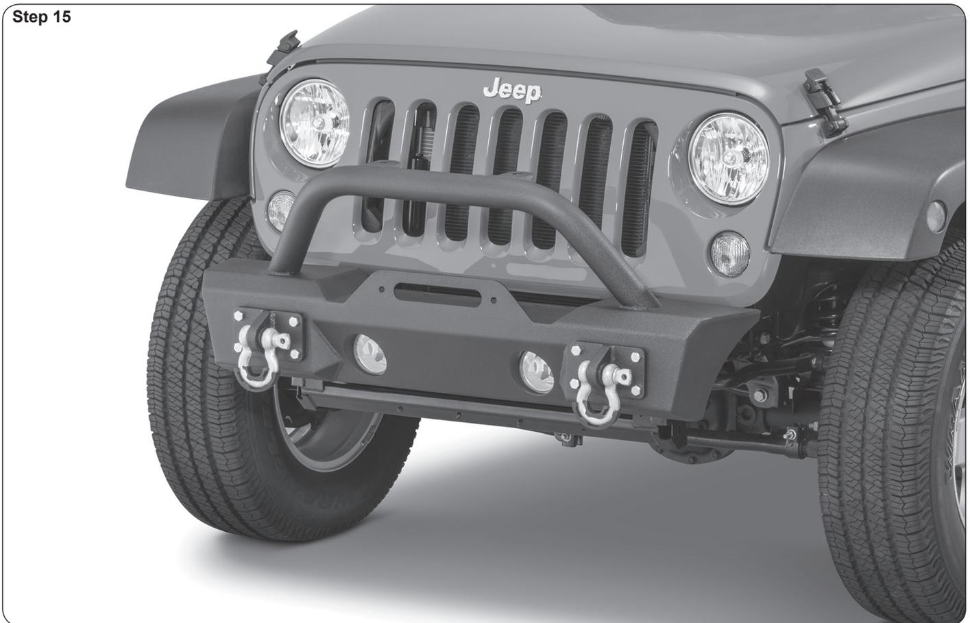
Finally, install D-Rings with provided washers and Isolators. (Step 15)
