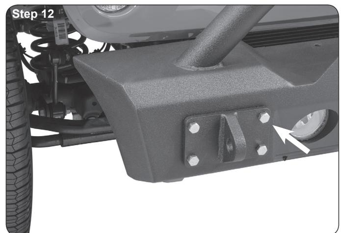
Pass 4 M12 bolts through the D-ring mounting bracket and through the factory frame holes. Repeat on other side. (Step 12)
