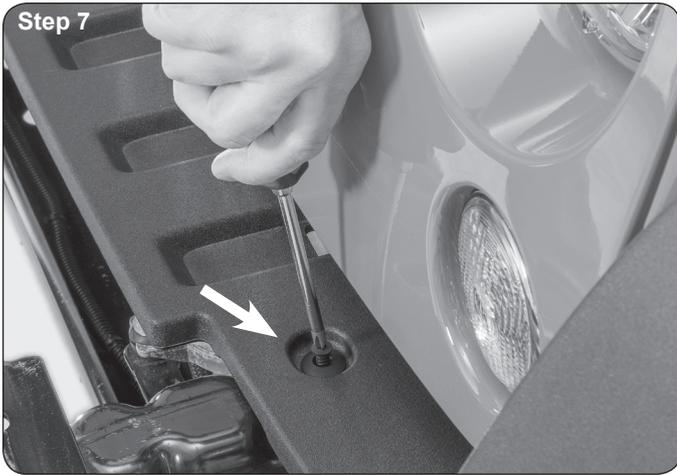
Remove the plastic screw rivets with a Phillips screwdriver. (Step 7)
