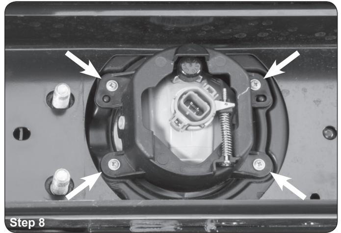
Remove the factory fog lights from the factory bumper with a Phillips screwdriver. (Step 8) Set aside fog lights for reuse later.
