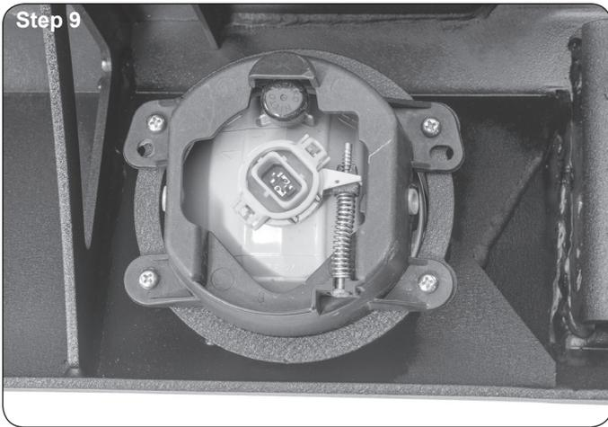
Install the fog lights with the 8 provided Phillips head screws and flange nuts using a Phillips screwdriver. (Step 9)
