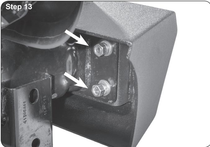
Secure the bolts with the 8 M12 nuts, split washer and flat washers on the back of the frame. Tighten with an 18mm socket and ratchet. (Step 13)
