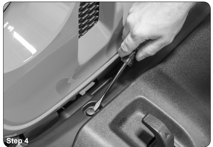
Remove the plastic retainers using a small flat blade screwdriver. (Step 4)
