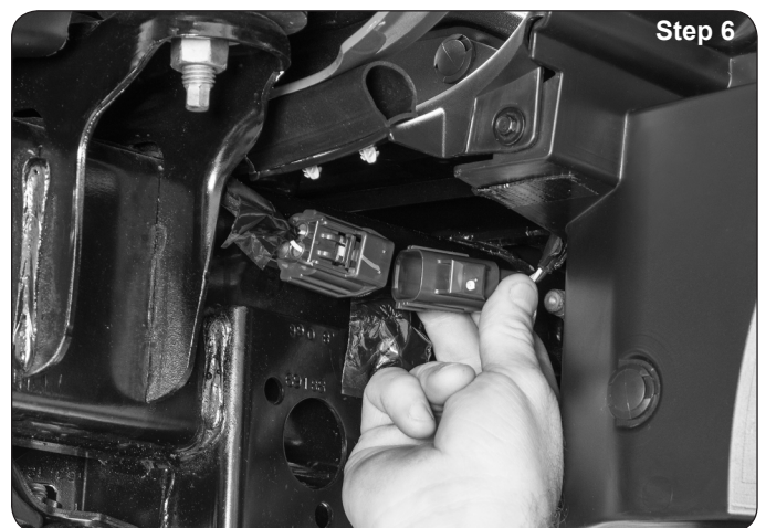
Disconnect the fog light wiring harness plug and remove bumper. (Step 6)
