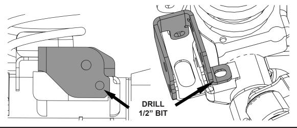
INSTALL ONE OF THE M12 BOLTS AND THE PROVIDED SERRATED NUT THROUGH THE BOTTOM. THREAD THE NUT ONTO THE BOLT FINGER TIGHT.
