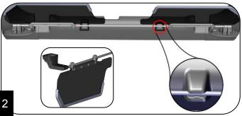
Install rod mount over the top of where the rod clips into factory visor support. Rod mounts have tabs on the back side that index onto the rod and into the Jeep's factory trim visor supports. Position mount and install the four Phillip's screws.
