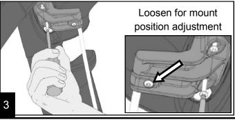
**Note:** The Axis Sun Visor has 2 friction setting bolts and 4 mounting bolts. The upper 4 mounting bolts (pictured) should be kept tight and not be loosened to adjust rotational stiffness. The lower two bolts can be tightened or loosened to adjusted for rotational stiffness.
