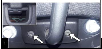
Next, install the left and right Axis Sun Visor Mounts, using the screws that were removed from the factory sun visors in step 1. **Note:** If holes do not line up, then loosen the right side rod mount bolt (1/8" hex bit) and adjust position of rod and mounts as needed. Once mounts are installed retighten rod mount bolt.
