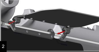
Flip the Axis Visor back up to access the under side of the mirror mount.
