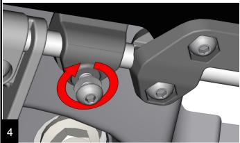
Once the bolts and washers are reinstalled into the mirror you can use these 2 bolts to tighten and loosen the rotational stiffness of the mirror.
