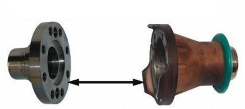
Measure from lip of flange on transfer-case out-put to face of flange at differential.
