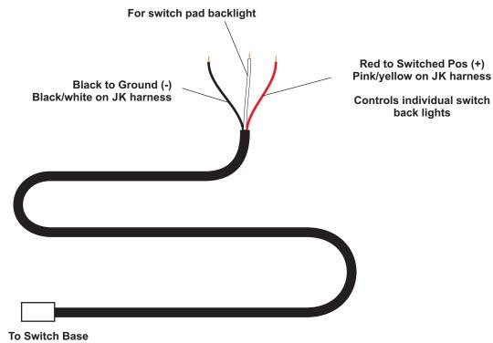
Wiring for the back lighting on the RF switch pad includes 3 wires for connection. The RED is used to back light the individual switches when they are turned on and should be connected to switched ignition (Pink/yellow on JK).
