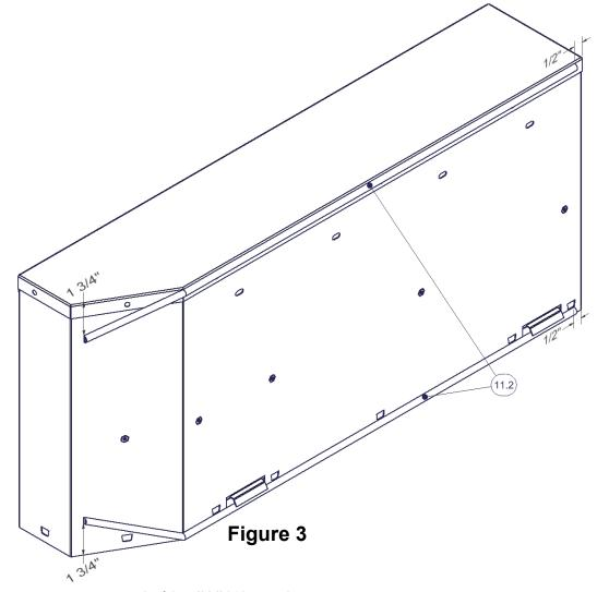
4. Separate the #11.2 Double D-Seal into two pieces (lengthwise) and apply them to the back of the 359 Lockbox as shown in Figure 3.
