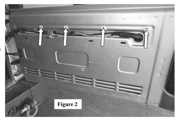
3. Install (4) #11.1 Plastic Inserts(found in the key bag) into the upper-right most holes, as shown in Figure 2.
