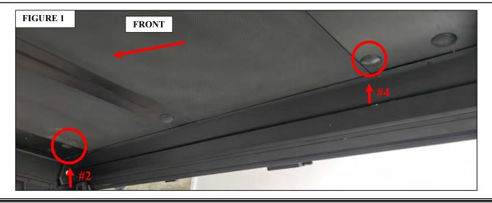
3. Remove the 2nd and 4th plastic plugs from the EXP Truck Cap Roof Panel, (Fig 2). Then remove the M6 Hex Nuts and M6 Flat Washers inside the plastic plugs, (Fig 3). Keep the M6 Flat Washers.
