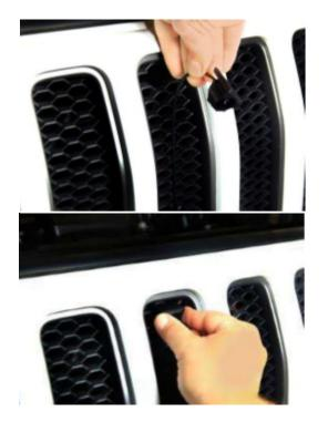
Insert the bottom tab into the grille, then snap the upper camera mount into place.
