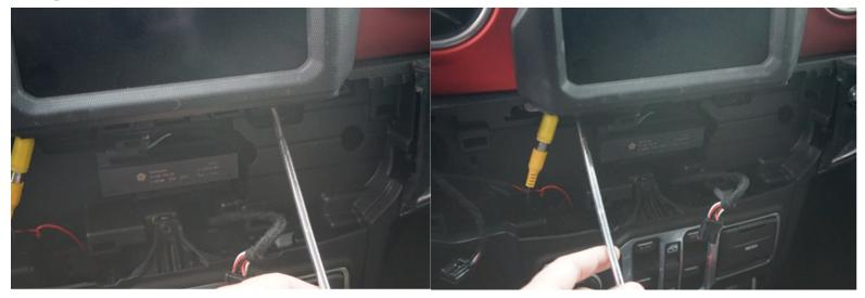
Using a Phillips head screwdriver, remove two screws holding radio bezel to dash.
