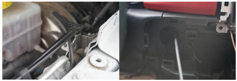
Using the wire routing diagram, run the camera wiring down the front of the vehicle and against the fender. The rear washer nozzle tubing hold down can be used to hold the camera wiring also. Run the wiring through the clutch plug and into the vehicle. Route under the dash and through the Push-to-Start wiring hole.
