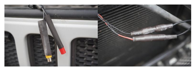
Place the included shrink tubing over one side of the camera connectors, then plug in the mating connector, making sure to cover both connectors with the heat shrink. Center the heat shrink, then use a lighter or heat gun to constrict the tubing over the connectors.
