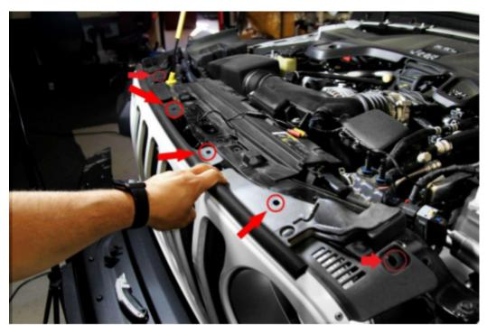
Remove the 5 clips holding the top of the grille to the core support. Once removed, you can lean the grille forward to aid in installation.
