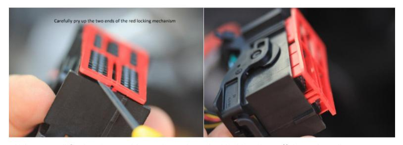
Using a small flat head screwdriver, raise red terminal locking plate off the main radio connector.
